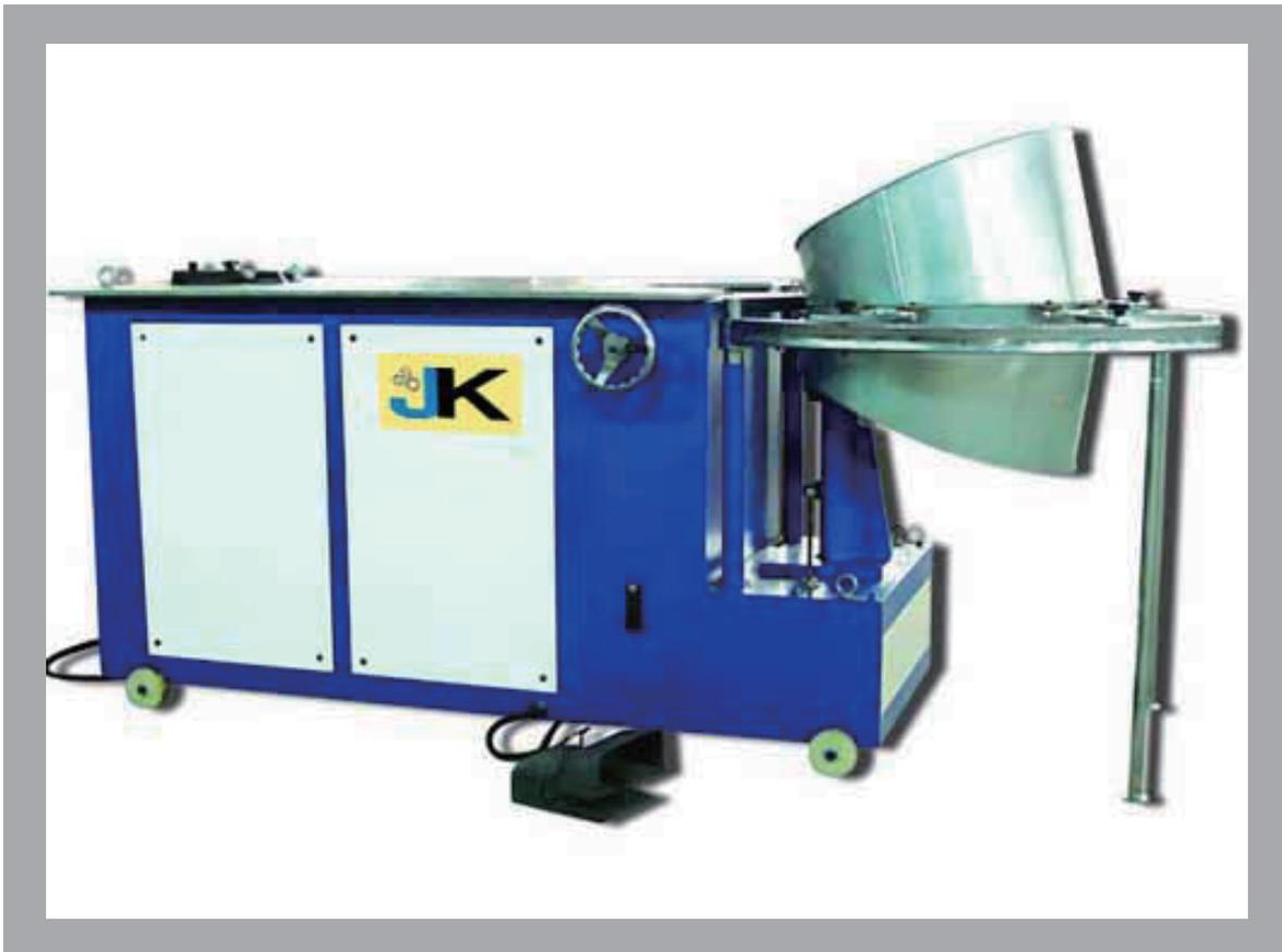
In HVAC duct work, the elbow is widely used for corners and turnings, the traditional manual work is heavy and noisy. You can easily make the elbow by this machine, without hard work and noise round your head. The Economy type is half automatic, which has dual head, can do the flange operation and seam locking at the same time(2 seperated motors)
