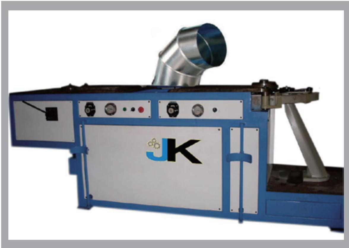
In HVAC duct work, the elbow is widely used for corners and turnings, the traditional manual work is heavy and noisy. You can easily make the elbow by this machine, without hard work and noise round your head. The Hydraulic type has 2 operation station and a higher efficiency which can make an 8" elbow in 90 seconds.
