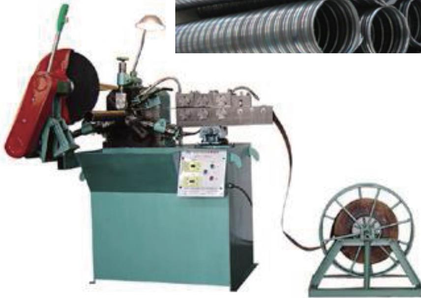
Spiral Corrugated Tubeformer is made for the concrete project, like the bridge building and other kinds of construction. CT78 is widely used in bridgeworks in and out board, which has a compact form and easy to transport. The spiral corrugated pipe machine can be taken to the construction site where the post tension pipe is needed.
