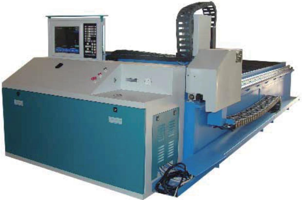
Plasma Cutter choose the industrial computer control system utilizes a MITSUBISHI servomotor system with industrial control software, the professional HVAC software from Lantek. To connect them, an advanced communication system and composing software are used. The most important unit is the plasma generator is from American Hypertherm or Thermal Dynamics.
