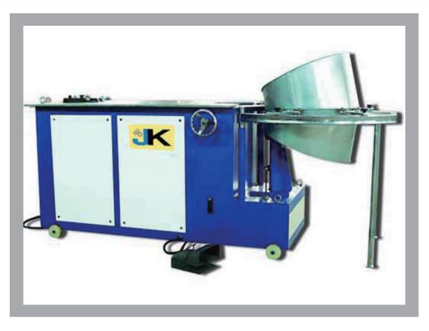
In HVAC duct work, the elbow is widely used for corners and turnings, the traditional manual work is heavy and noisy. You can easily make the elbow by this machine, without hard work and noise round your head. The Economy type is half automatic, which has dual head, can do the flange op -eration and seam locking at the same time(2 seperated motors)
