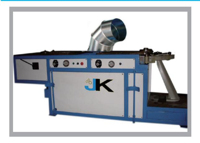
In HVAC duct work, the elbow is widely used for corners and turnings, the traditional manual work is heavy and noisy. You can easily make the elbow by this machine, without hard work and noise round your head. The Hydraulic type has 2 operation station and a higher efficency which can ma -ke an 8" elbow in 90 seconds.
