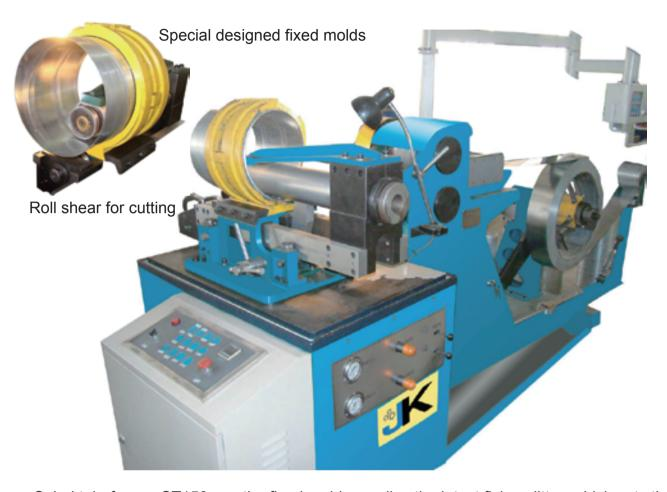
Spiral tubeformer ST150 use the fixed molds, applies the latest flying slitter, which cuts the tubes to length without noise or hot sparks as known from the saws and provides smooth tube ends without deburring.
