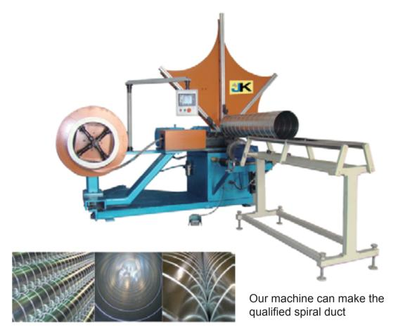
Spiral tubeformer ST80 has the largest diameter range from 80mm to 1600mm, and use the special steel tape molds, which can reduce the molds cost heavily. Also the automatic cutting system can easily set any length to cut and has the reliable performance. The most economic spiral duct machine.
